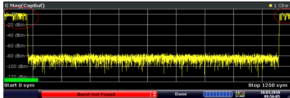
Figure 10-2: Example for incomplete burst capture
