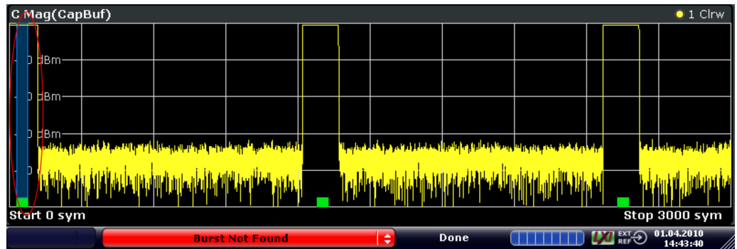
Figure 10-3: Example for measurement on incomplete burst capture
