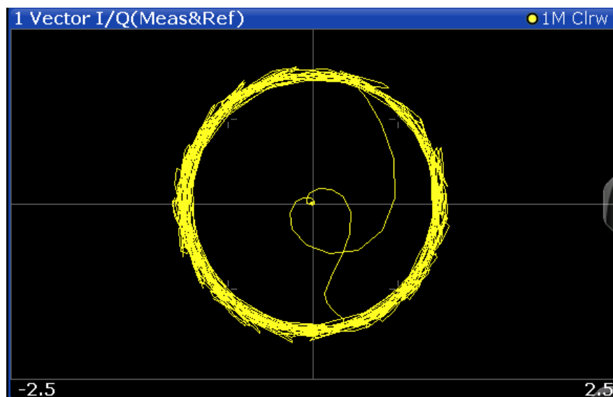
Figure 3-24: Result display for "Vector I/Q"
