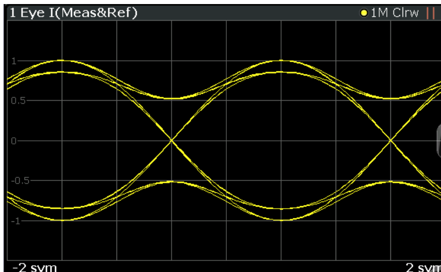
Figure 3-7: Result display "Eye Diagram Real (I)"
